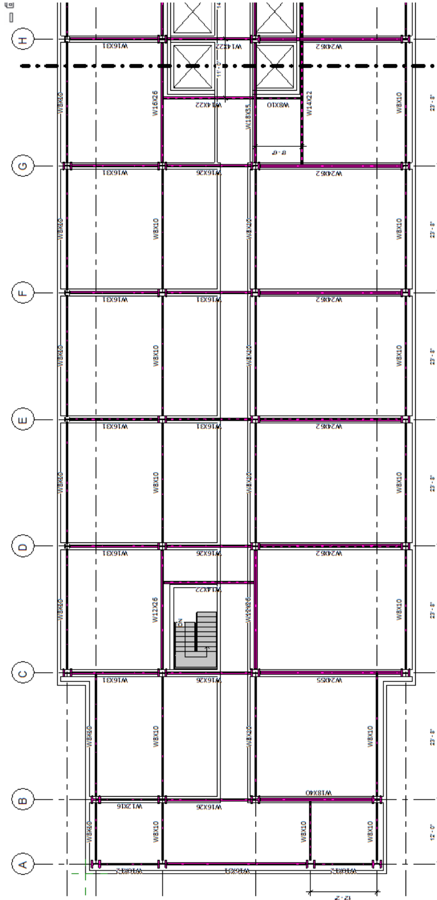
Figure F.2: Typical Framing Plan for Residential Levels of Proposed Design Note: Match line to Figure F.1
